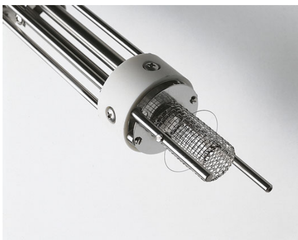
Figure 11: Analyzer head of an RGA. Its main components are an ion source, a mass filter, and an ion current detector (not shown). The ion source is built on the white ceramic terminal. Behind the terminal, there are four rods of the quadrupole mass filter between two supporting shafts. Courtesy of SRS Stanford Research Systems.
