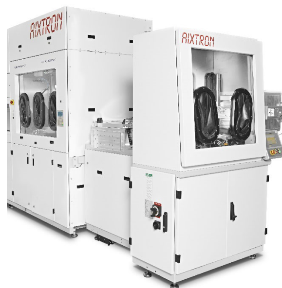
Figure 5: A section of a metal organic chemical vapor deposition system. The glove box on the left protects the reactor chamber from air during service, the glove box on the right is used to load and unload the substrates. With permission from AIXTRON SE.
